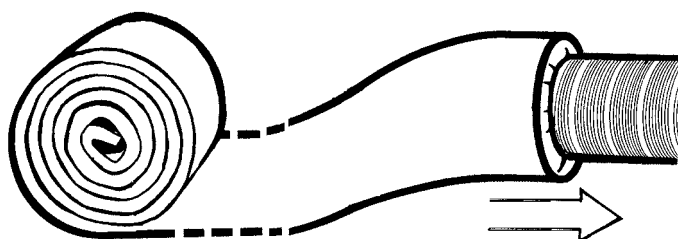
3. Unroll, slip the "hose" over the duct
